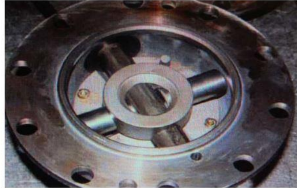
Figure 7 Drive long shaft past stub shafts
