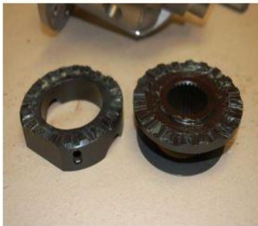
Figure 12 Coat Teeth of drivers, couplers, and washers with grease
