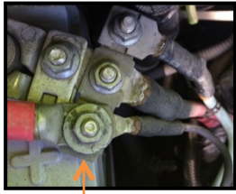
Positive side – 10mm socket
