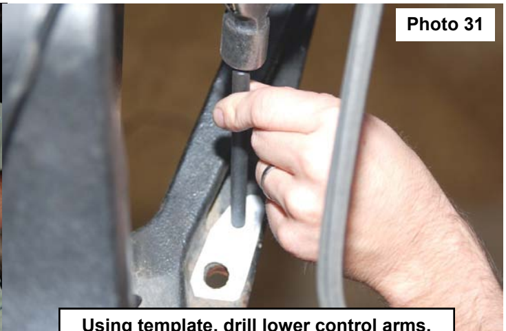
Using template, drill lower control arms.
