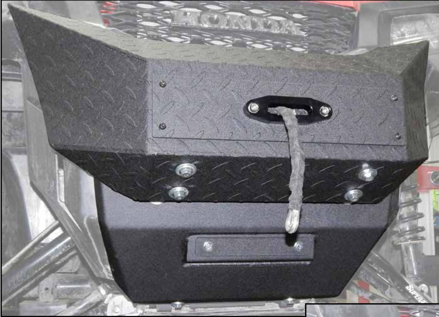
SuperATV 3500 Lb. Winch installed
