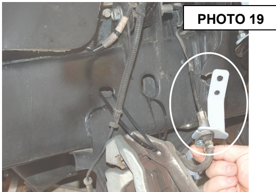
Install the line on the new bracket.
