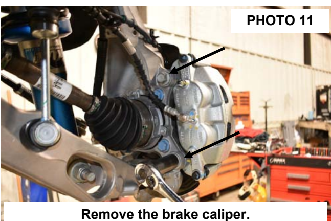
Remove the brake caliper.
