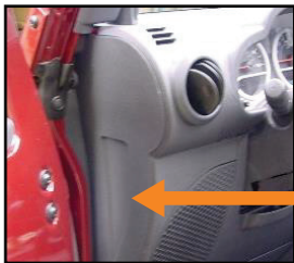
Use a small screwdriver and pry out plastic
