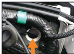
Use this hole on upper right side of brake booster
